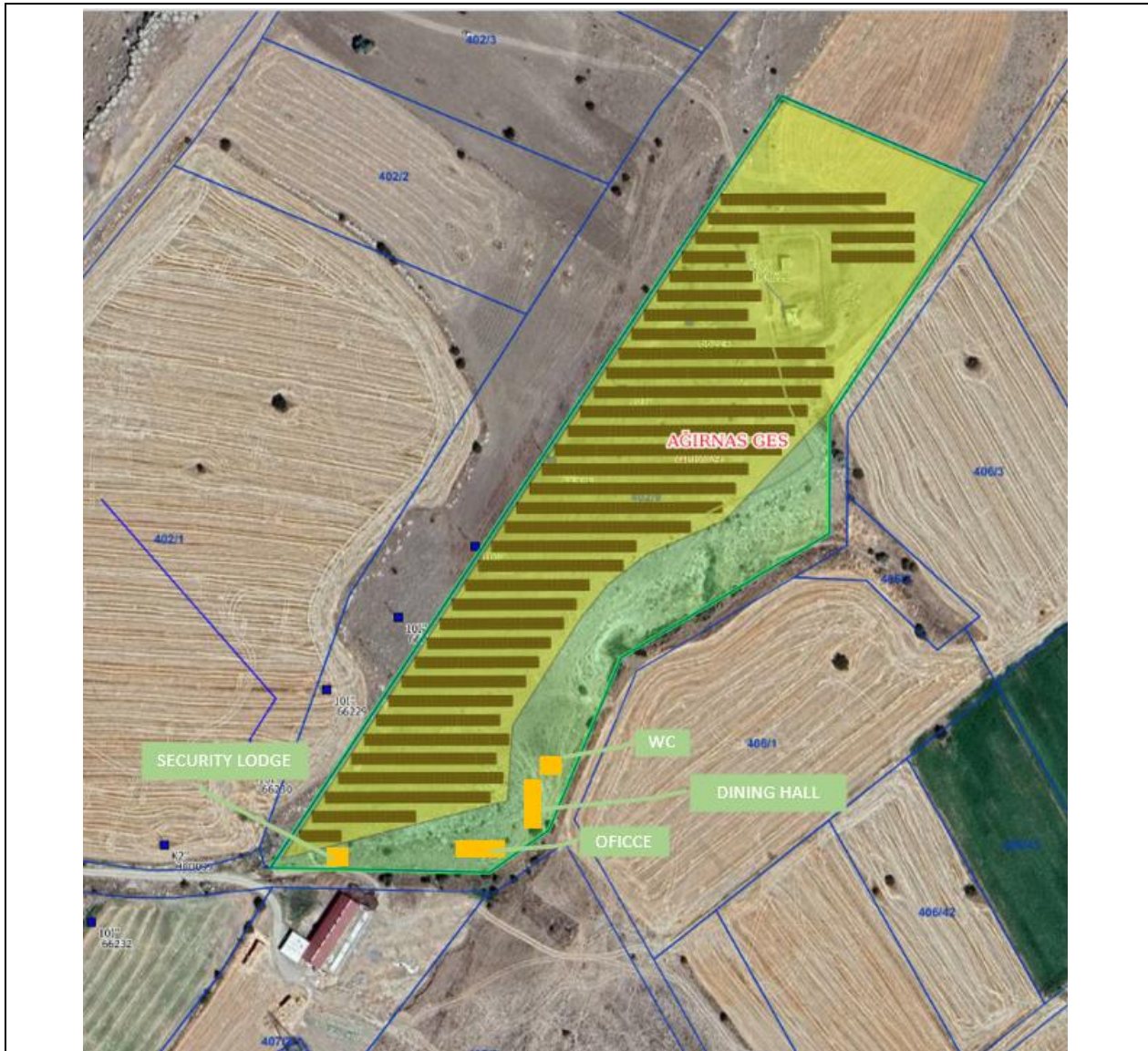
Figure 15 . Construction Camp Site Layout
